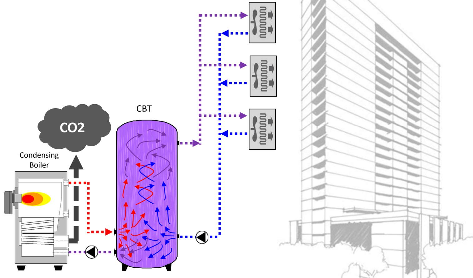
**NOTE:** In a PRIMARY-ONLY system CBT represents system hydronic thermal-mass with supply/return manifolds experiencing same mixing effect.
